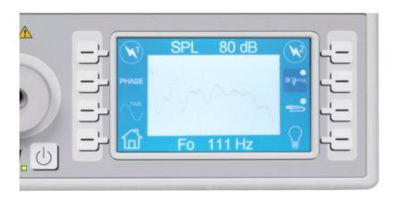
The angle of the LED flash in Phase mode (0-400°) can be modified through the powerful software and the pedal, as well as the flash speed in Slow motion (0.5-2Hz), providing hands-free operation.
